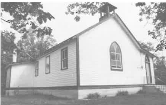
180) MacKenzie Presbyterian Church Construction Date: 1922 Location: River Lot #120 Present Owner: Presbyterian Church of Canada Present Use: Active Congregation Construction: walls - horizontal siding on milled wooden frame roof - asphalt shingles on milled wooden rafters Integrity: Largely unaltered Condition: Good
