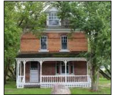
The house has original woodwork, doors, floors, banister and newel post. It received municipal designation in 1997 and since then, the roof was replaced and gutters and downspouts put in place, the brick re-pointed and the verandah rebuilt. It is currently owned by the City of Selkirk.
