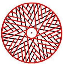
These images show the typical pattern cut into a millstone. The diagram on the right shows the kind of intricate patterns that were cut into the static bedstone and the moving runner stone in such, comparable to the action of hundreds of pairs of scissors when the runner stone was moving. The angle of the crossing lines tended to push the grain towards the outside of the millstones where the flour could be collected.
