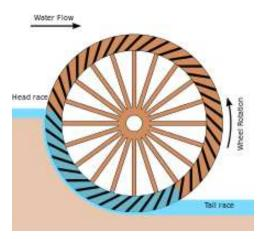
Breastshot water wheel, in which the flow of water is directed over the mid points of the wheel.
