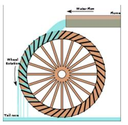
Overshot water wheel, in which the flow of water is directed over the topmost points of the wheel.
