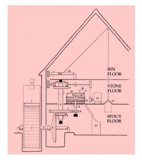
This image describes a more complex operation than obtained at John Gunn's mill, but it does provide a clear graphic sense of some key parts of mechanisms and of likely operations: the water wheel (2) on the large axle (3) turning the large gear (4) which engages other gears (5, 7 and 8) and finally the smaller axle (9) that turns the millstones (10 and 11). Different sizes of gears where used to gradually reduce and refine power levels to the grinding stones.
