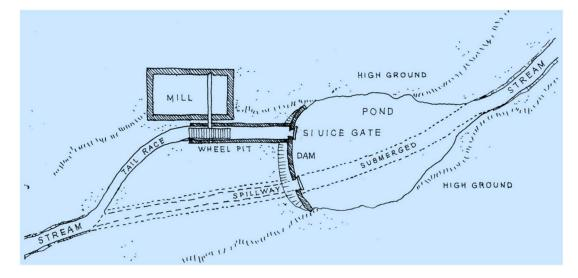
This sketch plan shows an imaginary mill situated on generally flat ground, and thus with a trench that is used to divert water from the main stream course. A sluice gate and bridge shown at the right-hand side were used to control water volumes that entered into the trench.
