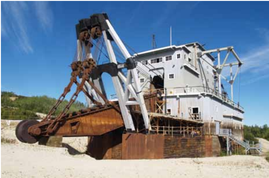
The deteriorated heavy timber bow gantry frame of Dredge No. 4, in Dawson City, YK, was dismantled and replaced in kind with a new frame, built from new timbers sized to match the original timbers and reusing all original metal brackets and fixtures. The bow gantry, which supports the digging ladder, is a significant constructed element in the dredge's operational design.
