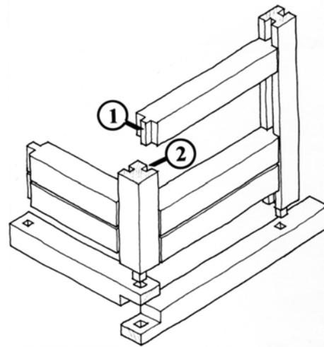
Top: A typical small log cabin. Above: A cut-away detail showing Red River frame log construction (1 is the tongue and 2 is the tenon). Below: A cut-away detail showing a dovetailed corner.
