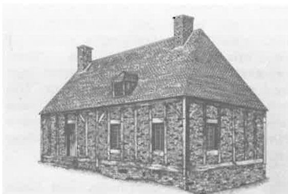
Plate 12. "Maison en columbage", a very common construction procedure used in New France during the seventeenth century (From: Building a House in New France , p. 24.)
