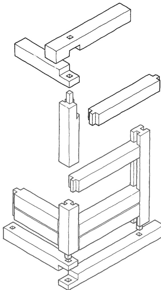
Plate 14. Construction procedures of Red River frame.
