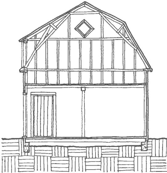
Plate 95. Cross section A-A of the Charaton barn.
