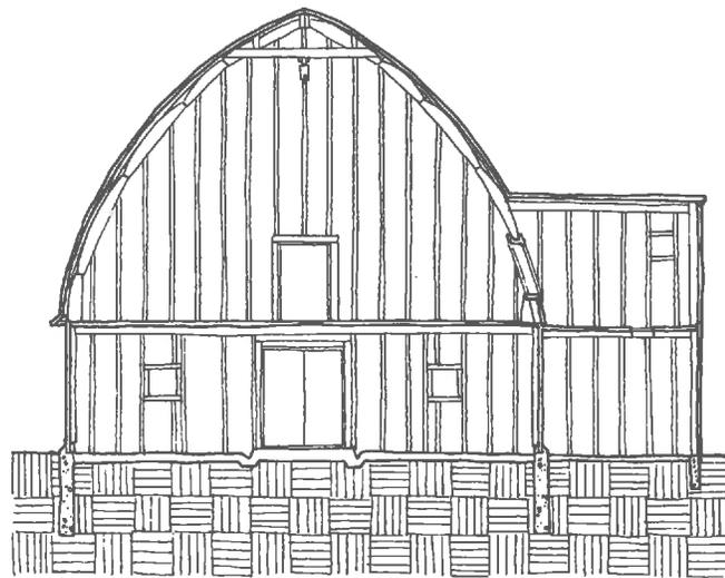
Plate 97. Cross section A-A of the Jenkins barn.
