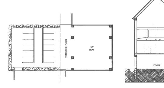
Plate 68. Stable and loft plans (superimposed) and section of a bank barn.
