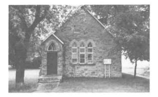
189) Garson Mission Church Construction Date: 1919 Location: Garson Present Owner: Baptist Church of Canada Present Use: Active Congregation Construction: walls - solid fieldstone roof - asphalt shingles on milled wooden rafters Integrity: Largely unaltered Condition: Good Notest This building is also discussed on page 125.
