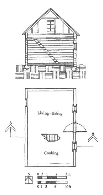
Plate 71. Section A-A and, below, plan of the Hawkins house.
