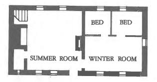
Plate 33. Plan of a typical French stone cottage. (From: <u>Cottages of Quebec</u>, p. 9.)
