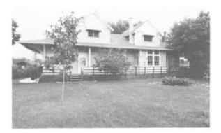
237) Former Petersfield Rail Station Construction Date: 1929 Location: NE 23-15-4E Present Owner: Mr. Houghton Present Use: Residence Construction: walls - horizontal siding on milled wooden frame roof - asphalt shingles on milled wooden rafters Integrity: The interior has been renovated for its current function Condition: Good
