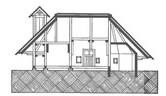
Plate 164. Section through a Bukovynian church. (Redrawn from materials prepared by the Manitoba East European Society.)
