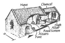
Plate 50. The parts of a small medieval church shown with the fabric cut open. (From: Architecture in Scotland, p. 52.).
