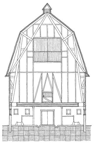
Plate 89. Cross section A-A of the Overwater barn. The loft floor is unnecessarily strong, built of two layers of 40x200s.
