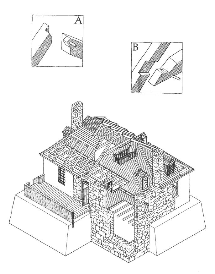
Plate 42. Isometric cut-away of the Bunn house and details of the rafter apex (A) and the rafter brace (B). Some of the earth surrounding the house has been removed to reveal the lower extent of the stonework.
