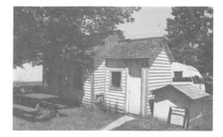
156) Summer Kitchen Construction Date: ca.1915 Location: 423 Sinclair Avenue, Selkirk Present Owner: Mrs. L. Morriseau Present Use: Storage Construction: walls - horizontal siding on milled wooden frame roof - wood shingles on milled wooden rafters Integrity: Unaltered Condition: Good
