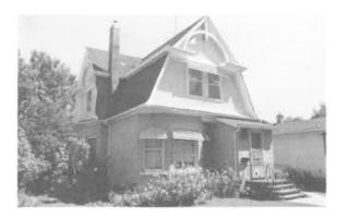
22) 1 1/2 Storey Side Hall House with Gambrel Roof Construction Date: 1905 Location: 215 Rosser Aveue, Selkirk Present Owner: Mrs. Ellen Howard Present Use: Occupied Construction: walls - horizontal siding on milled wooden frame roof - wood shingles on milled wooden rafters Integrity: Largely unaltered Condition: Good
