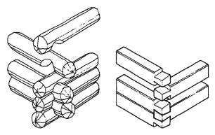
Plate 69. Saddlenotch and dovetail corner joints.
