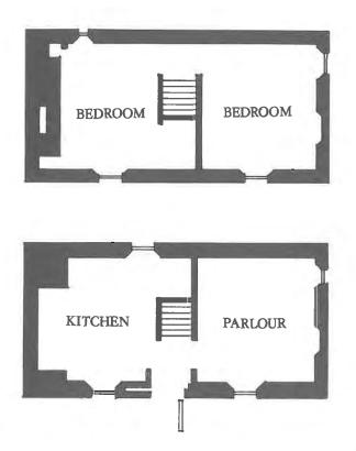
Plate 31. Plans of a typical laird's house.
