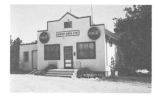
228) Newman's General Store Construction Date: ca. 1920 Location: SW 19-16-8E Present Owner: Mr. Newman Present Use: Vacant Construction: walls - stucco veneer on milled wooden frame roof - asphalt shingles on milled wooden rafters Integrity: Unaltered Condition: Good Notes: This building is also discussed on page 105.
