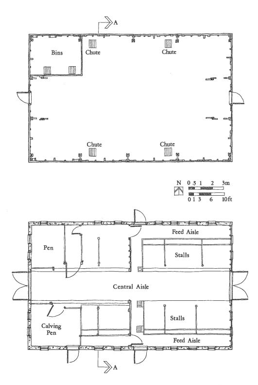
Plate 90. Loft plan, above, and stable plan, below, of the Overwater barn.
