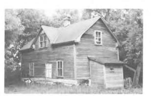
78) 1 1/2 Storey Central Gable House Construction Date: ca. 1890 Location: NW 36-17-3E Present Owner: Mr. N. Swirski Present Use: Occupied Construction: walls - horizontal siding on milled wooden frame roof - asphalt shingles on milled wooden rafters Integrity: Largely unaltered Condition: Fair
