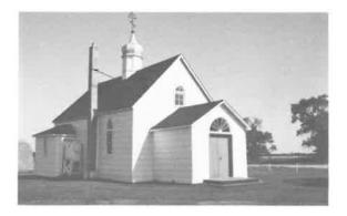
Ukrainian Orthodox Church of the Holy Trinity Construction Date: 1906 206) Location: SW 27-15-6E Present Owner: Ukrainian Orthodox Church of Canada Present Use: Active Congregation Constructions walls - horizontal siding on milled wooden frame roof - asphalt shingles on milled wooden rafters Integrity: Largely unaltered Condition: Good
