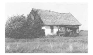
57) Galician Log House Construction Date: ca. 1920 Location: Present Owner: Mr. Sawchuk Present Use: Abandoned Construction: walls - plaster veneer on square dovetailed logs roof - wood shingles on squared logs Integrity: Largely unaltered Condition: Poor
