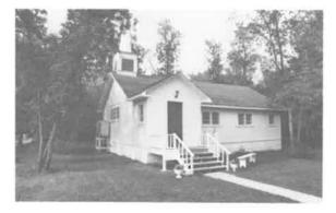
176) All Saints Anglican Church Construction Date: 1922 Location: Whytewold Present Owner: Anglican Church of Canada Present Use: Active Congregation Construction: walls - horizontal siding on milled wooden frame roof - asphalt shingles on milled wooden rafters Integrity: Largely unaltered Condition: Good
