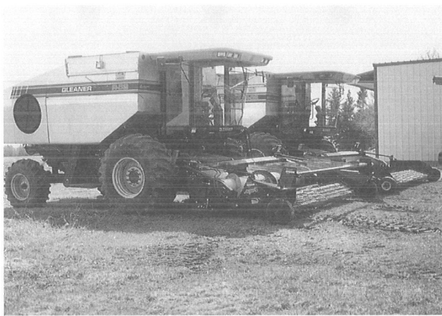
Gleaner R62 Combine – Capable of harvesting 4 – 5000 bushels of wheat or 8000 – 10000 bushels of barley in one day. Engine size is 260 HP., grain tank 300 bushels, fuel tank is 150 gallons, 16 hrs of continuous running.
