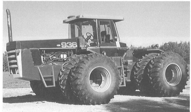
Versatile Tractor Model 936 – Cummings Engine producing 325 HP – Traction – 4 wheel drive, having dual tires. Some models have triple tires.
