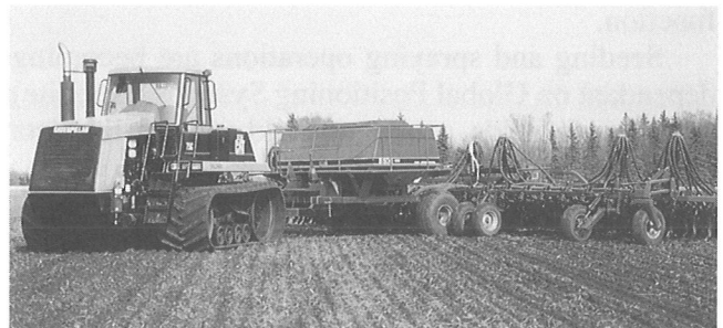
Caterpillar 75 C Tractor running on a continuous 35 inch wide rubber track, also producing 325 horsepower. The advantage of the track is mainly compaction and less slippage. – Air seeder has 7 inch spacings and covers 45 feet in a pass. Capable of seeding 300 acres in one day. Some newer models are 70 feet in width.
